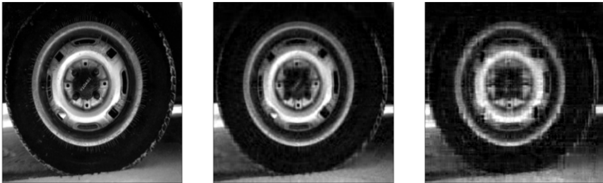
Figure 1: Tire image compression (a) original, (b) SVD approximation, (c) CLS approximation, t_{max} = 100 .
